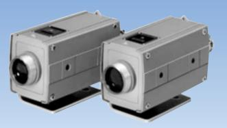
The KL(R)50 Series sensors are through-beam type CMDs that output ON-OFF signals by detecting blocking of light by the detected object that passes between the transmitter and receiver.
